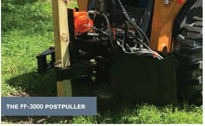
The "right tool for the job" comes down to efficiency. After the PP-3000 for guard rail post, Amkin applied the design to mini skid steer units for landscaping and fencing projects. The PP1800 makes quick work of the removal. For shrubs and trees the vibrating effect removes the dirt from root ball to eliminate waste. No more digging, no more straps.
